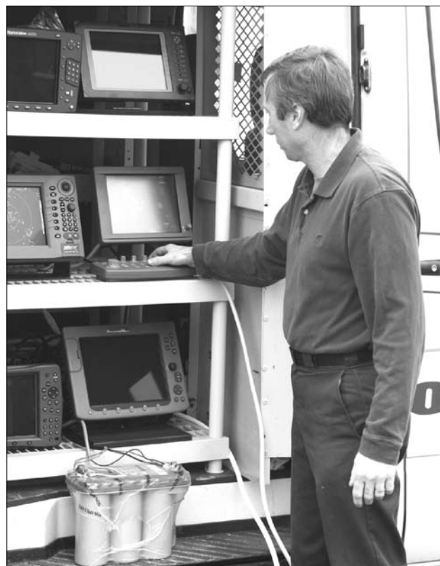
Above: Performance tests were based in large part on how well each radar showed shoreline 15 miles away and a few lobster pot floats about a half-mile away.
