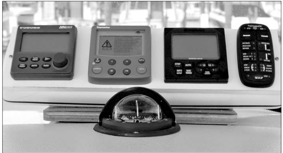
Above, from left: Furuno (Navpilot 511OB), Raymarine (ST6002+G), Simrad (AP16VF), and Nautamatic TR-1 Gladiator. Right: All were tested on a 26-foot center console.
